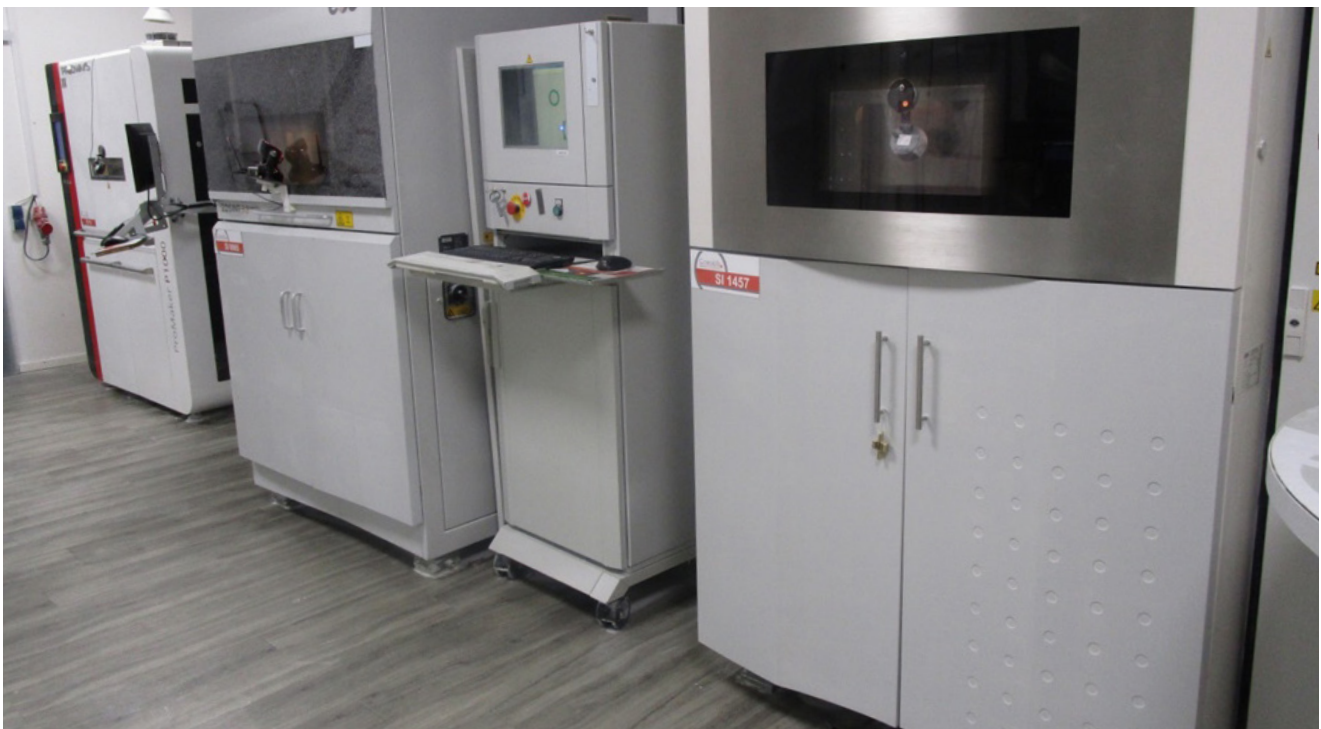
A battery of SLS systems at Creabis, including both Prodways and EOS technology
