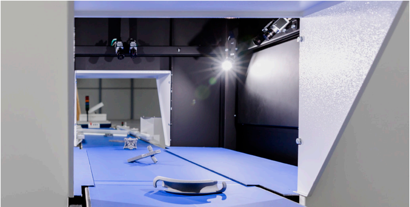
Identifying parts in a split of a second with vision technology based on their geometry only
