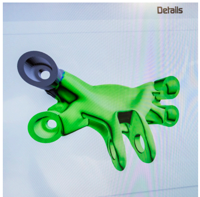
Comparison of point cloud with the digital source files showing missing details on the parts in grey.
