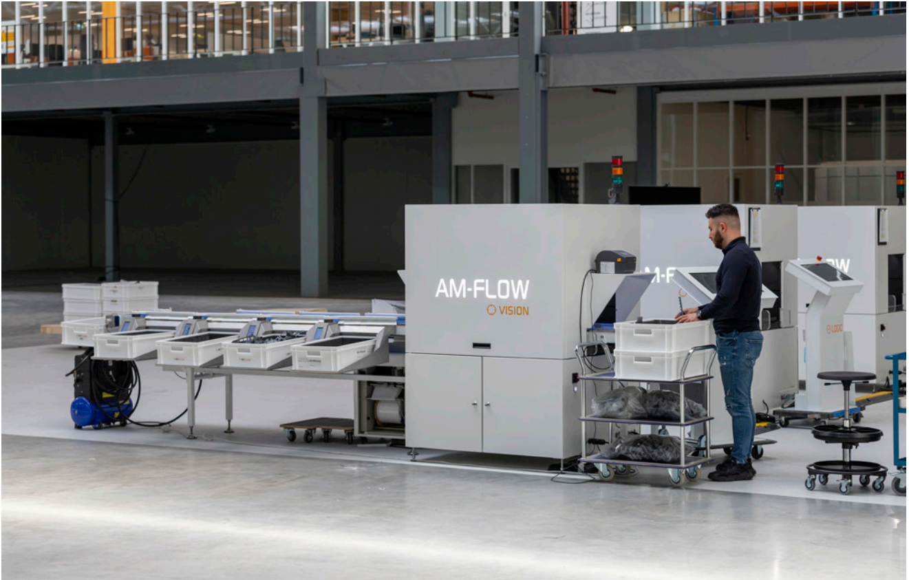
Basic set-up for identifying and sorting 3D printed parts with the AM-VISION and AM-SORT
