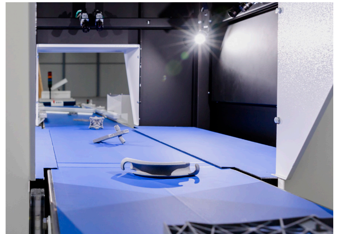
The AM-VISION automates part identification using cameras and intelligent software to match printed parts to their STL files.
