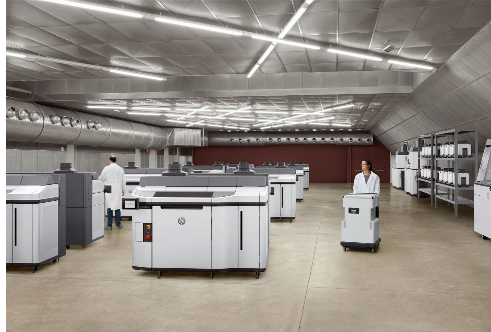
HP's MJF systems were developed to be highly automated in combination with post-processing units for part cooling, powder handling and powder recycling. 15
