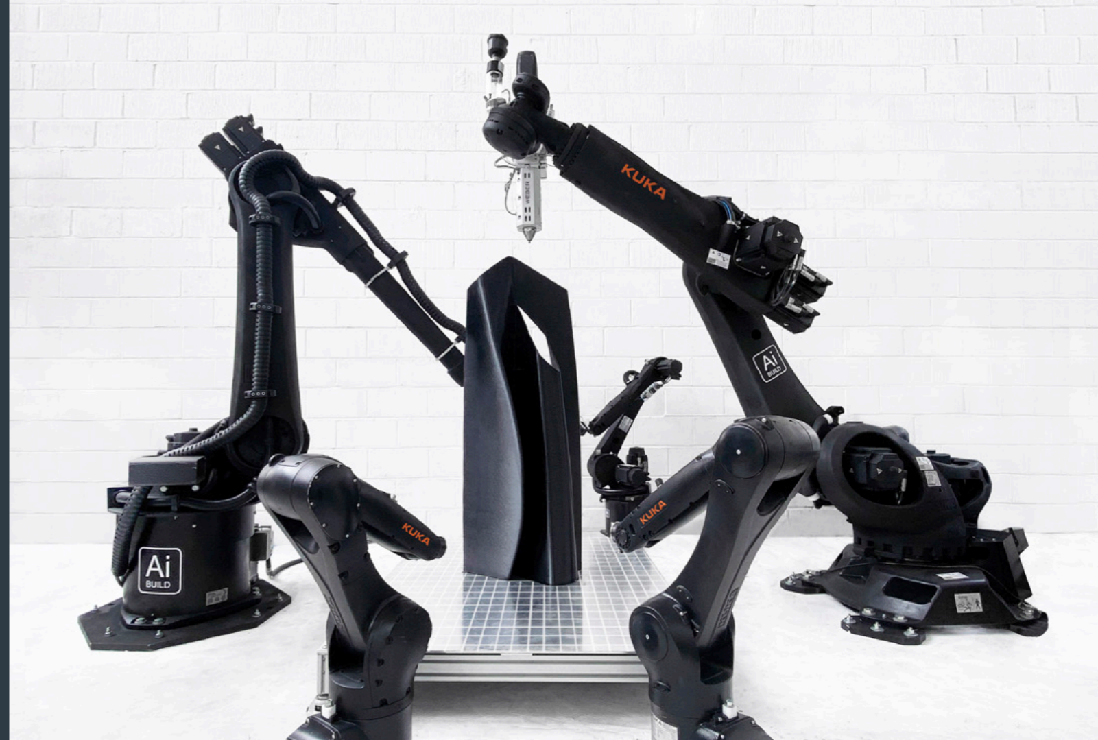
Ai Build's autonomous additive-subtractive robots manufacturing a jig for a Formula E race car. 8
